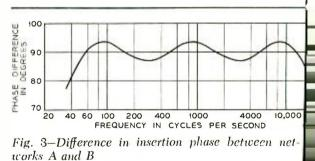
and a phase-shift network is also inserted in the carrier supply to one of the modulators marked A in Figure 1. The network in the signal branch to the A modulator shifts the phase of all frequencies by 90 degrees plus an angle,  $\theta$ , which varies with frequency, while the network in the branch
