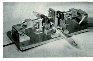
Fig. 8—Lead wire soldering tool with a plate holder containing an EDT crystal plate, with disks alreadyattached, in center position. This tool, by interchangeable noses, is also used to attach the combination adhesive disks to the plate. Each headed wire registers in accurate alignment on its corresponding disk and is soldered in a radiation heat cycle for minimum thermal stress
