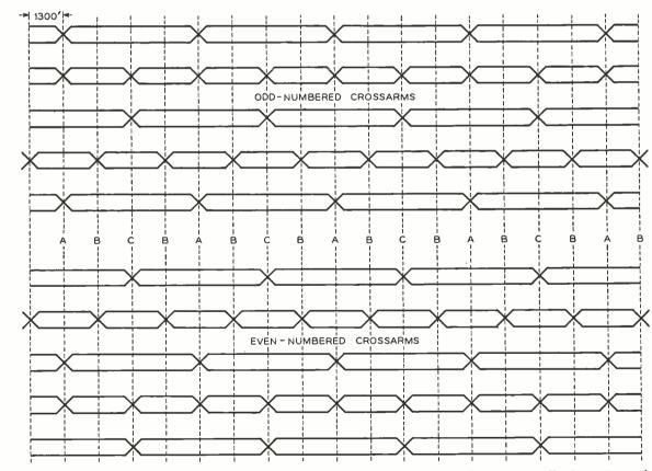
Fig. 1–The ABC transposition system, shown above, was the first to result commercially from Barrett's invention
