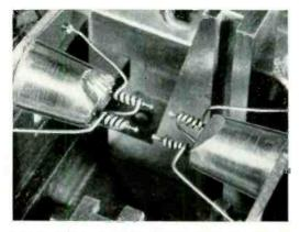
Fig. 9—Close-up of lead wire soldering tool to show details of soldering noses. The fixture provides for soldering all four wires to the disks simultaneously
