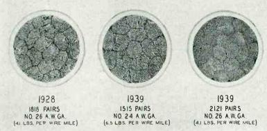
Fig. 3—A pictorial survey of full-sized Bell System exchange cables from the first paper-insulated lead-sheathed cable of Barrett's to the 2121 pair cable of 1939. Cables in the two bottom rows are 2% inches outside diameter
