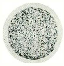
Fig. 2—Cross-section of 100-pair, No. 19 gauge, dry-core paper-insulated cable of 1892, with an extruded lead sheath
