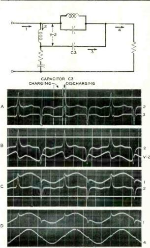
Fig. 5–Oscillograms of currents and voltages in harmonic generator network. Numbers at right indicate points at which measurements were made
