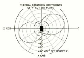
Fig. 5—Thermal coefficients of linear expansion in directions parallel to the major face of a Y-cut EDT crystal plate. The negative Y-axis extends toward the reader
