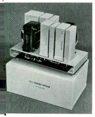
Fig. 1–The 103A frequency generator resting on the case in which it is housed when in use
