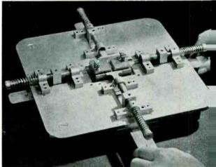
Fig. 7–Centering tool for positioning an EDT plate inside its holder
