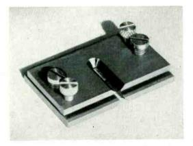
Fig. 6—An EDT plate holder in which plates are friction held. It accommodates any size of plate up to  $1\frac{1}{2}$  inches in length,  $1\frac{1}{4}$  inches in width, and 3/16 inch in thickness, provides the mechanical protection needed by the plate, and insures a more uniform heating and cooling rate to minimize plate fracture from thermal heat
