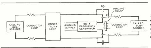
Fig. 2-Method of applying ringing current to the called line and audible ringing to the calling line
