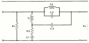
Fig. 3-Circuit of the 103A frequency generator
