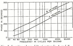
Fig. 2-Insertion phase shift of networks A and B
