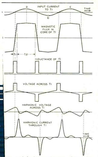
Fig. 4-Idealized curves of current, voltage, and inductance referred to in the description of audible ringing generation
