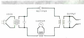
Fig. 1–A simple circuit employing a rectifier as a modulator
