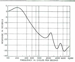
Fig. 3-Relative calibration curve of a search tube transmitter. Through use of a simple equalizing network the sensitivity may be made reasonably independent of the frequency in the range shown
