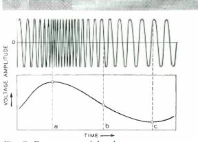
Fig. 5–Frequency-modulated waves represent t variations on the pattern by variations in frequency
