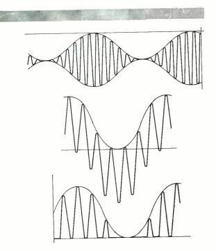
Fig. 2-Modulated wave (above) with two methods of demodulation-Heising method (center) and rectitying method (below)
