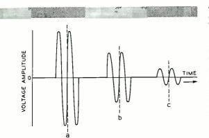
Fig. 7-Amplitude-modulated waves carrying pulses
