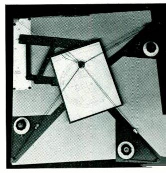
Fig. 2 - A 65-mc impedance plotting board. For clarity the three cords, upper left, are separated
