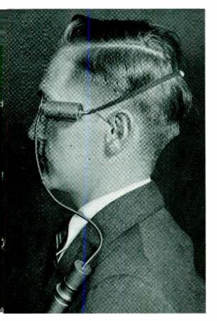
Fig. 2-Experimental equipment for sound pressure measurements in the auditory canal, modeled by S. Balashek. A spectacle frame and headband support the microphone which is connected to the preamplifier on the left shoulder. The search tube is bent to enter the ear canal and the seal of the telephone receiver is not appreciably broken by the tube. Duplicate equipment is used on the right side for binaural measurements
