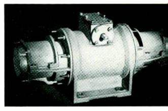
Fig. 5-The waveguide phase shifter with the drive shaft by which the  $\Delta 180$ -degree section is rotated
