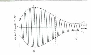
Fig. 4—The amplitude of the waves is modulated to bear the imprint of the pattern in Figure 2
