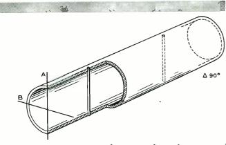
Fig. 2–Transverse conducting rod used to control velocity of wave in guide
