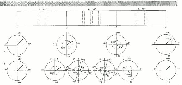
Fig. 4–Phase positions at input and output of the three sections of the phase shifter when the rods are all parallel, on A, and when the  $\Delta 180$ -degree section has been rotated 15 degrees clockwise, the vectors for the same input phase will be as shown on line B
