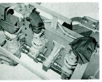
Fig. 6-A series of phase shifters connected by a common drive shaft as installed on an actual antenna
