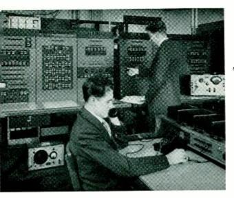
Fig. 2-The circuit simulator panels at the rear and a terminal position in the right foreground
