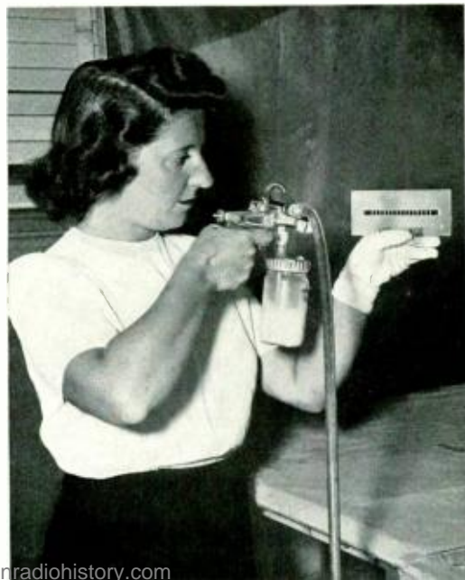
Fig. 4—Blanche Russiello spraying cathodes for the 396A
