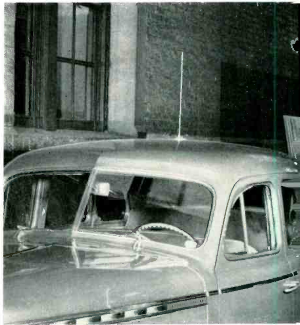
A short length of piano wire serves as the antenna for the mobile unit
