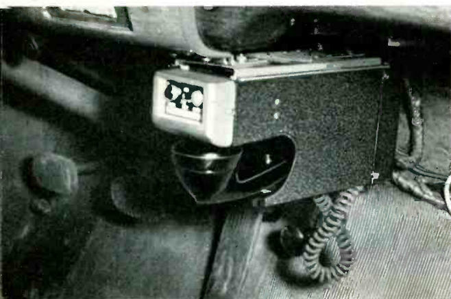
The vehicle control unit may be mounted under the dashboard or wherever most convenient
