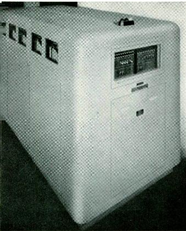
Closed view of the position table showing control panel and pilot lamps on top above it
