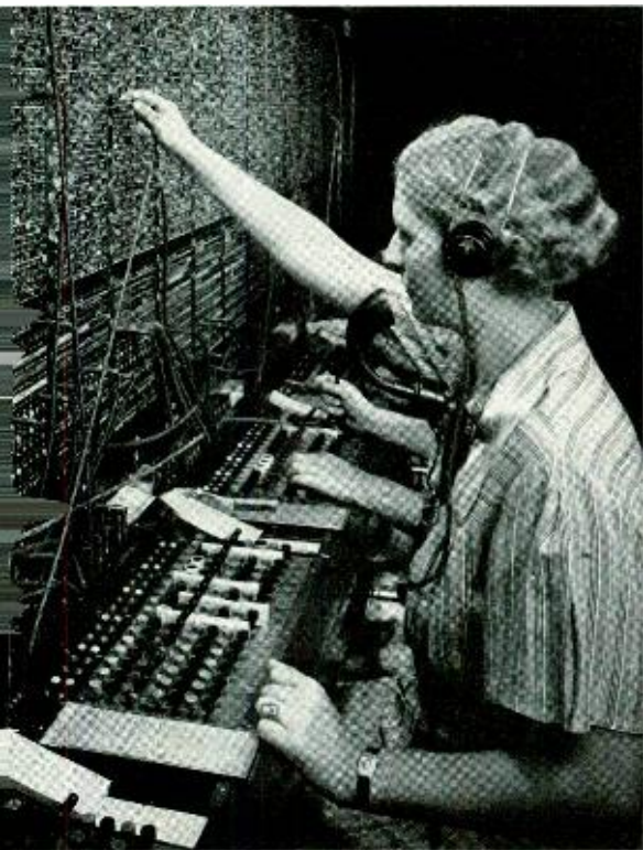
A No. 1 local manual board, not equipped for dialing or key pulsing
