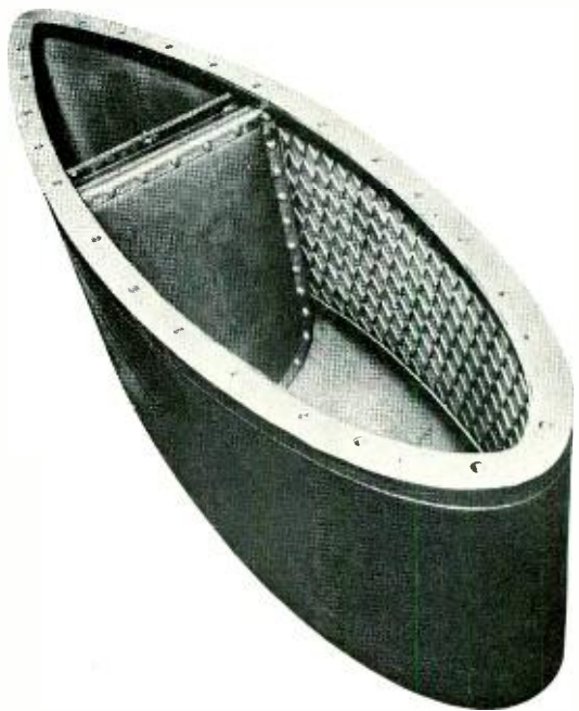
The stainless steel streamline dome of the QJA is transparent to sound over most of its surface
