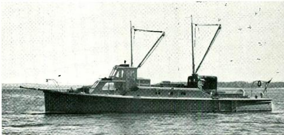
The Elcovee—Floating Test Laboratory for studies of sonar systems
