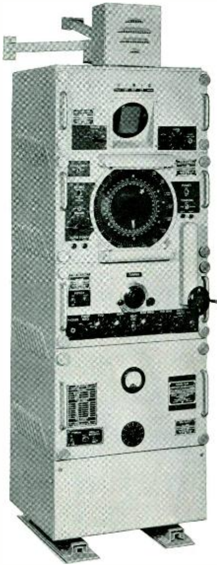
Control equipment rack of the QJA system
