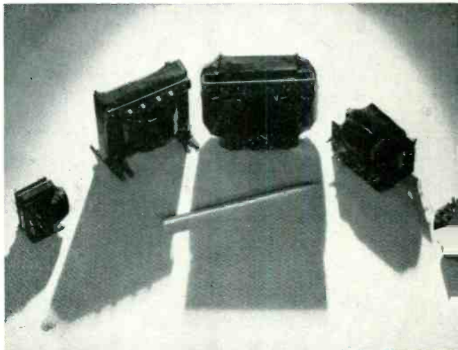
A row of encased, potted coils, hermetically sealed, and designed for ground and shipboard use
