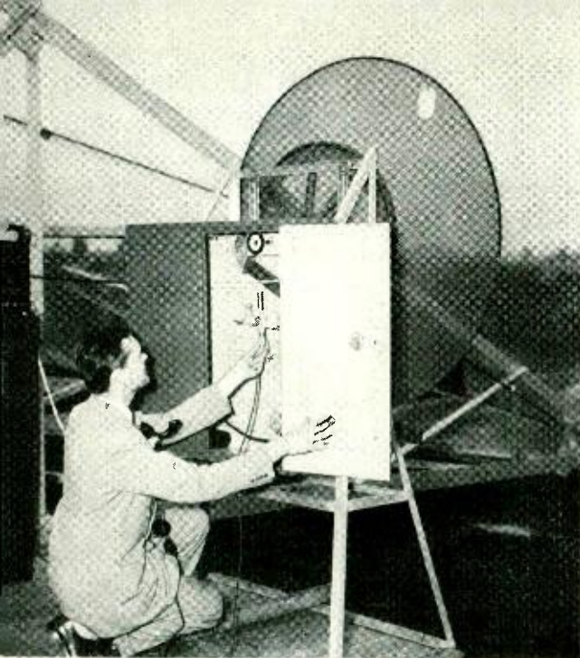
G. W. Atkins at the transmitter of a TE-1 radio television transmission system
