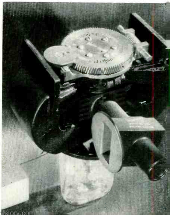
A three-centimeter magnetron (Western Electric 2J51) with integral magnet and tuning gear (shown at the top)
