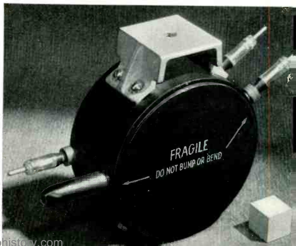
The first magnetron produced by the Western Electric Company. This is the 700A operating at 45 centimeters
