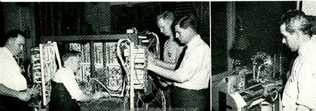
Assembling and wiring of a unit at Chambers Street shop (left)—Winding potentiometer cards for a gun director (right)
