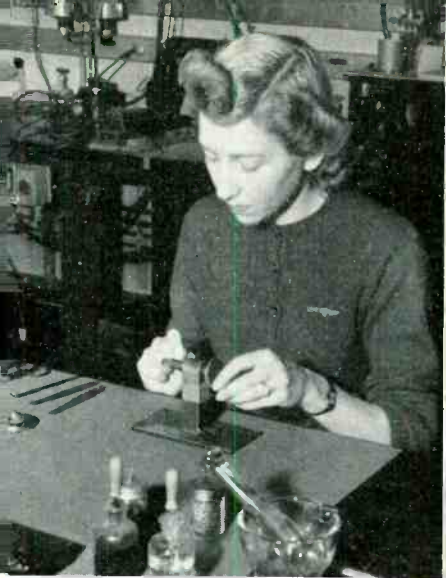
Winding fine wire for thermistor unit (left)—Assembling coils and transformers at the West Street building (right)
