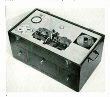
Fig. 3—Soldering machine designed for making wiresupported crystals
