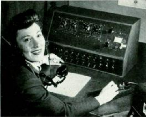
Radio instructor's desk of the crew trainer. This represents a control tower, or a squadron leader, or other planes in the flight
