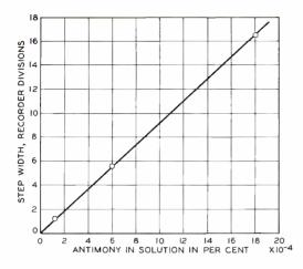
Fig. 4—Graph showing the relation between step width of the polarogram and the concentration of antimony in the solution
