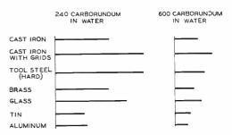
Fig. 2—Relative lapping speed of quartz with various materials for the lap
