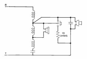
Fig. 1—Simplified circuit for the non-amplifying arrangement
