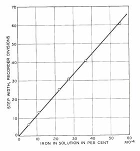
Fig. 5—Concentration of iron in solution in terms of the width of the polarogram steps April 1944
