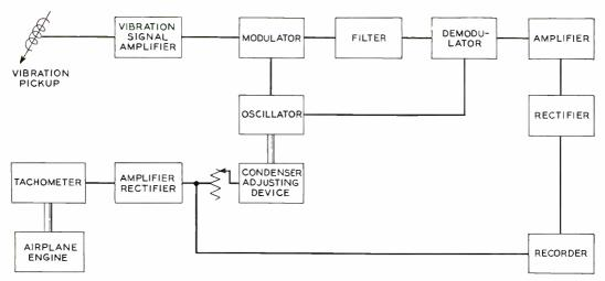
Fig. 2—Block schematic of analyzer circuit
