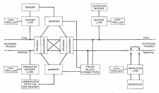
Fig. 2—Block schematic showing the main circuit components of the crossbar toll system April 1944 357
