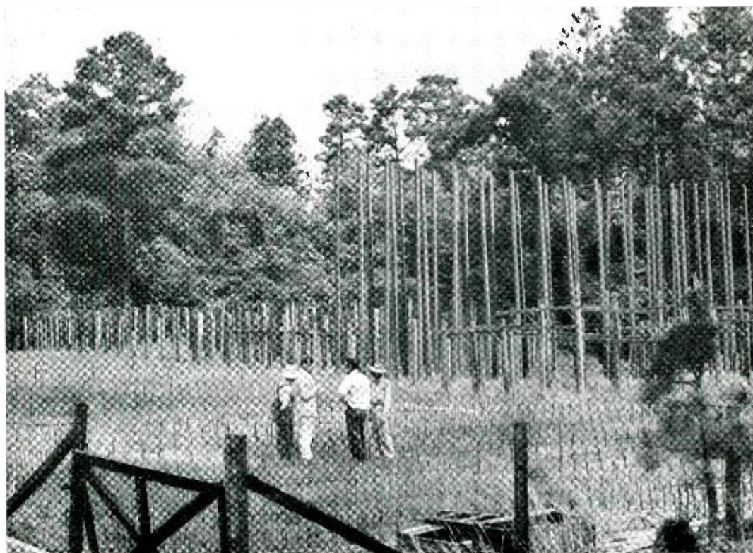
A section of the test plot at Gulfport, Mississippi, which shows square sticks under exposure test in the foreground and larger posts and pole-size experiments in the background
