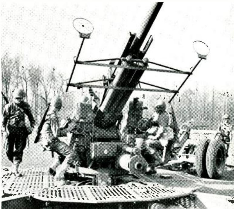
Gun pointers at each gun are standing by in case of need, but the motor-drives do the work under remote control of the Director
