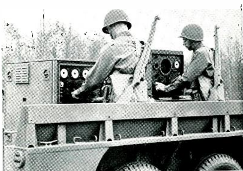
In the computer (left) data from the tracker and in the altitude converter (right) are combined with other information and the resulting electric currents are used to control the guns
