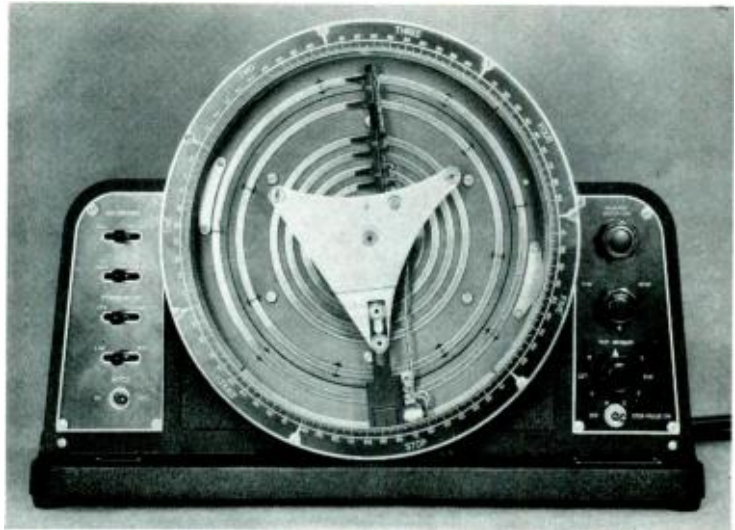
Fig. 3—Teletypewriter signals are transmitted through two segmented rings over which brushes rotate. Adjusting the outer ring with respect to the inner one determines the amount of signal distortion. Rings for the neon lamp are nearest the center
