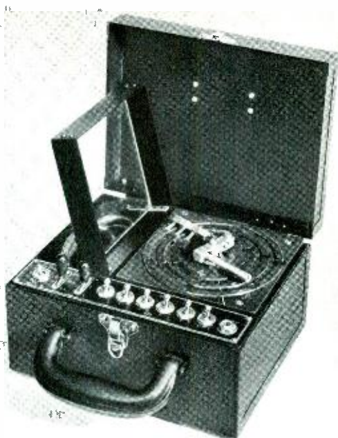
Fig. 7—The 100A teletypewriter test distributor is used primarily to check telegraph lines from subscribers' premises to the central office. The distortion produced is fixed at 20 per cent. It sends current reversals, for circuit testing, as well as distorted signals
