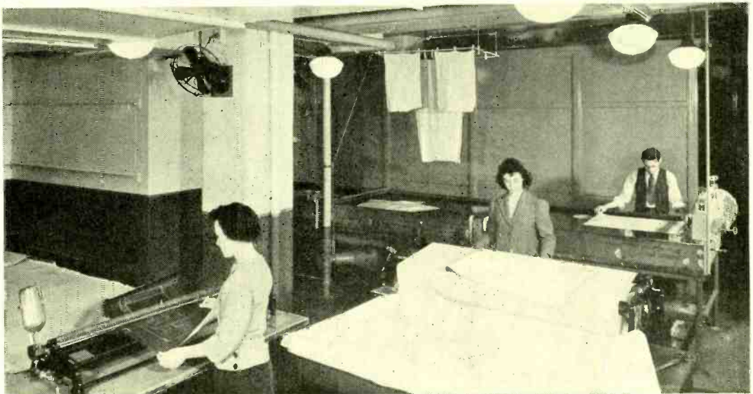
Fig. 5—After final washing, negatives are dried on the power-driven machine at the right and then passed through the oiling machine at left
