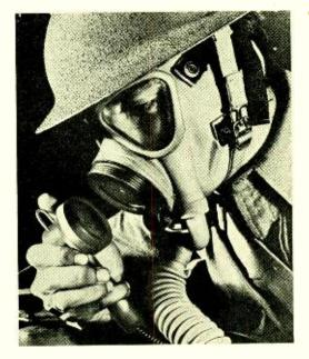
The Western Electric Microphone held in the soldier's right hand is widely used not only in field intercommunicating systems but also for radio communication between aircraft, tanks and their ground stations. There is a push-totalk switch in the handle
