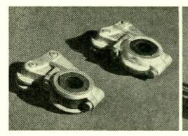
Fig. 2—A new bearing for vertical drive shafts of selector frames has a rectangular opening in its cap (left) to provide flexibility which prevents it from distorting the bushing. The rigid cap (right), formerly used, sometimes caused the relatively soft bushing to bind onto the shaft
