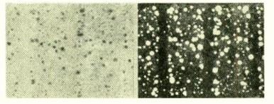
Fig. 1—Photographs of condenser paper broken down by acid liberated from the impregnant: (left) illuminated by ordinary light, (right) with ultraviolet light
