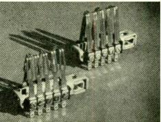
Fig. 3—Bifurcated springs are used in an improved assembly (left). The springs are clamped by a screw and can be changed separately. Previously the entire pileup (right) had to be removed and reassembled; all the connections also had to be unsoldered and resoldered
