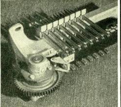
Fig. 4—The timing pulses from interrupters have been made more accurate by sturdier construction and by improving the cams and roller assembly
