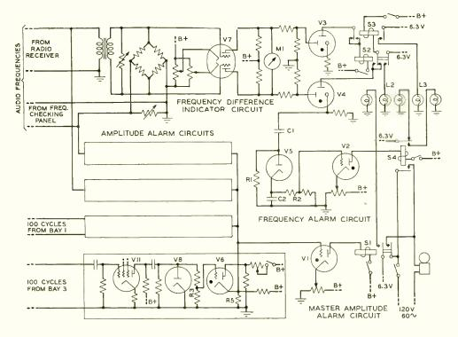
Fig. 2—Alarm and comparison circuit
