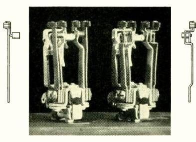
Fig. 1—Selector brushes with flexibly mounted shoes (right) cause less circuit noise than those with straight springs (left). The outside springs of the older type are straight while those of the new type have a U bend near the shoes
