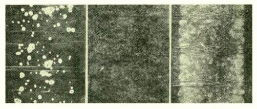
Fig. 2—Effect of exchange capacity of condenser paper on its service life. The two samples at the left were subjected to the same life test conditions at 120 volts. The linen paper (left) shows many decomposed spots scattered throughout the sample but Kraft paper (center) shows only slight evidence of decomposition. When the voltage was increased to 400 volts the Kraft paper (right) began to decompose
