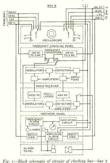
1000-cycle frequencies are carried to the indicator panel, where the difference is indicated, and gives an alarm if it exceeds a given amount.
