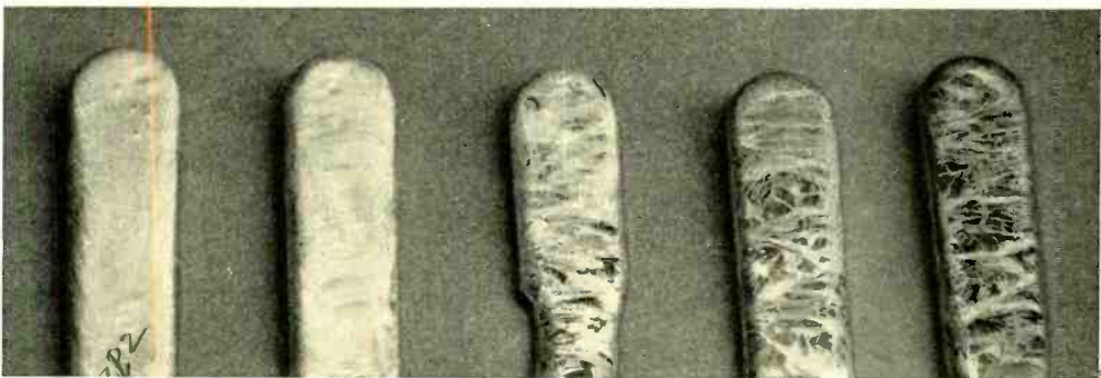
Fig. 2—The surface of test ingots becomes progressively duller and fissuring is more pronounced with increasing calcium content. From left to right these ingots contained from .021 to .030 per cent calcium
