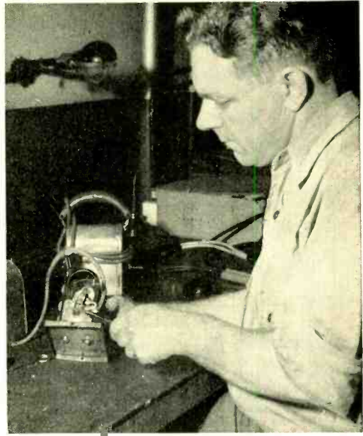
William Ruhe, an electrician in the Building Shops, repairing a watchman's magneto
