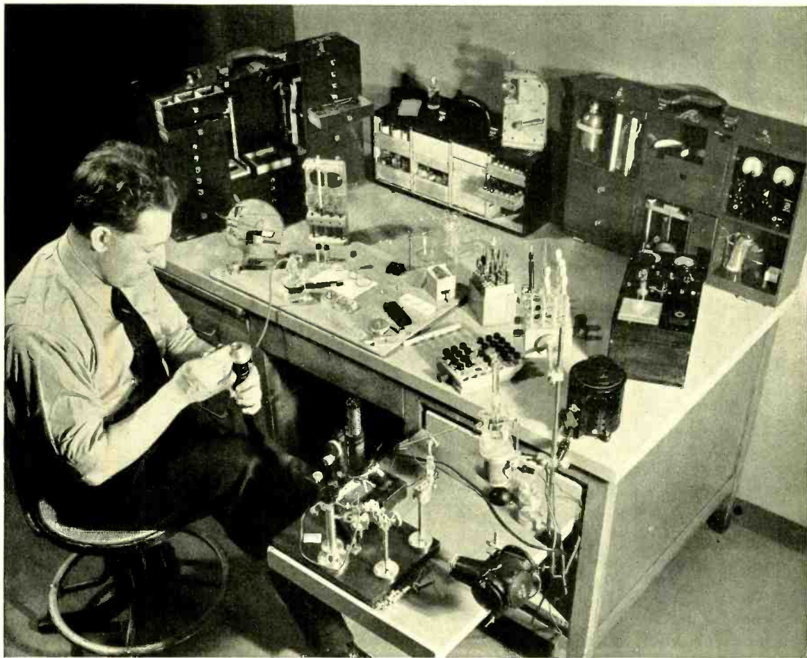
Portable microchemical equipment for investigations in the telephone plant
