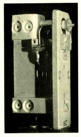
Fig. 1—The 9A reproducer is very small. Its diamond stylus is at the base of a T lever with minute coils on each arm
