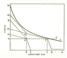
Fig. 4—Force-displacement diagram for clutch with release spring
