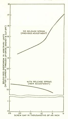
Fig. 3—Brush overtravel for various screwgap openings with and without the spring
