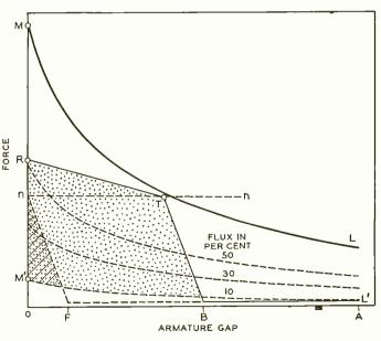
Fig. 5—Force-displacement designed for original clutch with a series of curves to show decreasing magnetic force
