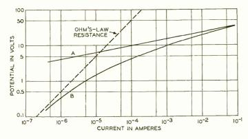
Fig. 4—Curves of Figure 2, when rearranged, show clearly that high resistance varistors depart more from Ohm's law than do ones of low resistance
