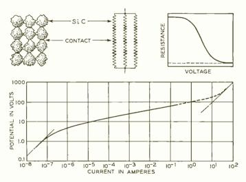
Fig. 1—Electrical characteristics of granular silicon carbide
