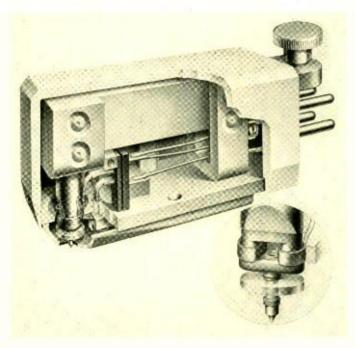
Fig. 2—The two pick-up coils are wound on a duralumin cup. A flat triangular spring between these coils supports them and the stylus. This spring flexes readily up or down but not sideways because of the wide cross section of the coils, thus restricting all motions except the lift required for vertical reproduction and the rotation of lateral reproduction
