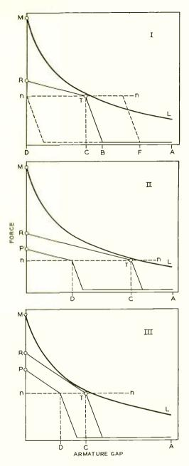
Fig. 2—Force-displacement diagram for the original clutch for various conditions
