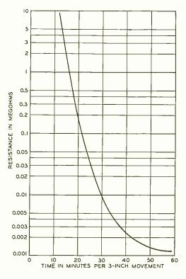
Fig. 3—Resistance of the varistors of Figure 2, measured at 20 volts and plotted against length of heat treatment
