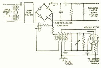
Fig. 3—Simplified schematic of the modulator circuit
