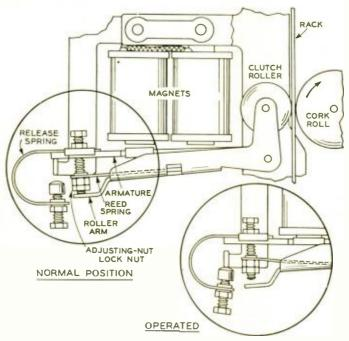
Fig. 2—.1 clutch equipped with release spring to provide a releasing force regardless of the screw-gap opening
