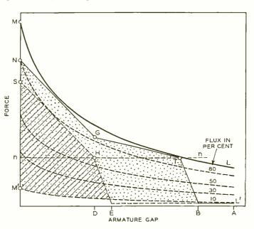
Fig. 6—Force-displacement diagram for clutch with release spring with a series of curves to show decreasing magnetic force
