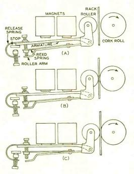
Fig. 3—Diagrammatic representation of the clutch with release spring—open position, above, and fully operated position, below
