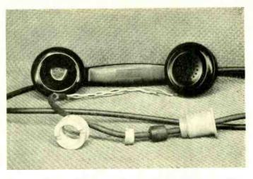
Fig. 5—The handset is connected to the housing by a rubberinsulated cord through a rubber-sealed clamp
