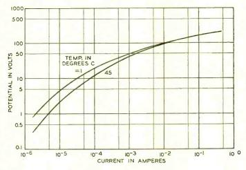
Fig. 7—For the same voltage, current approximately doubles with increase of temperature from 1 degree Centigrade to 45 degrees Centigrade
