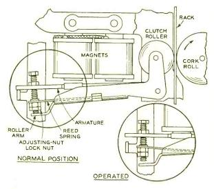
Fig. 1—Arrangement of clutch showing reed spring and adjusting screw
