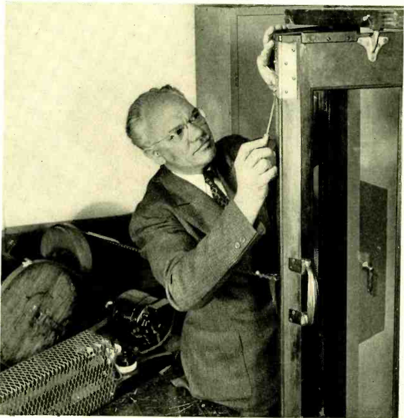
In making a life test of the door hinges of a telephone booth, the door is opened and closed repeatedly by a motor-driven mechanism until the hinges wear and the door fails to close completely. W. A. Krueger is shown inspecting a hinge for looseness
