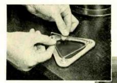
Fig. 1 (left)—A triangular frame with sliding pins in each corner is used to apply tension to the magnetic specimen
