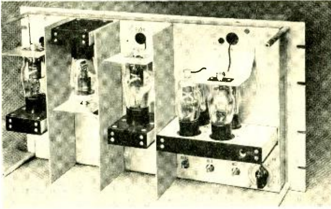
Fig. 3—The 1000^{-1} amplifier employed on the original experimental coaxial line
