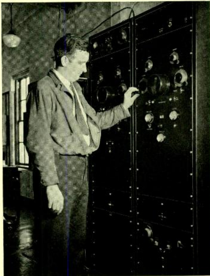
Fig. 1—The complete single-sideband receiver is housed in a single steel cabinet which is about twenty inches in width
