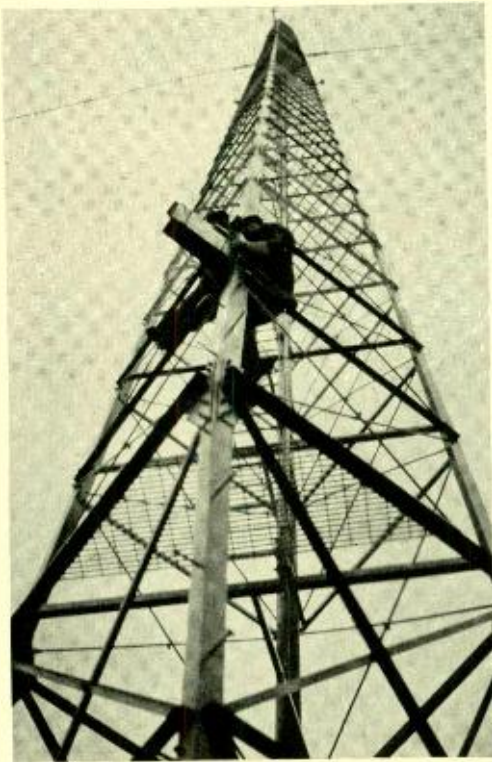
Fig. 8—To measure current distribution, a small loop was carried vertically up and down one corner of the antenna
