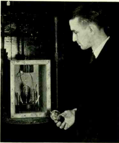
Fig. 1—The noise level of vacuum tubes is tested by carefully shielding them from electrical disturbances and mounting them on a spring suspension to eliminate vibration
