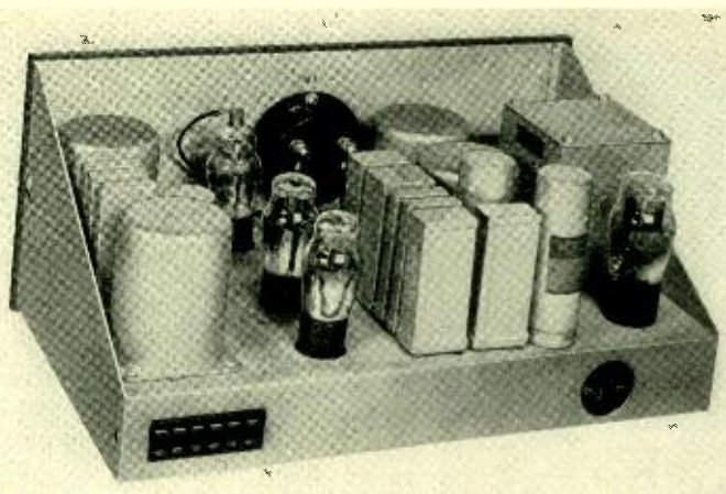
Fig. 2—Apparatus for the 89A amplifier is mounted on a metal chassis which may be readily removed from the cabinet
