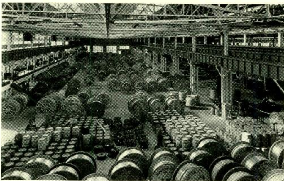
After being sheathed the cable is allowed to cool before being inspected and then crated for shipment
