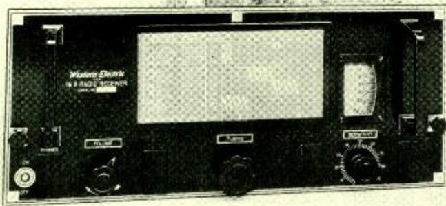
Fig. 4—Front view of direction-finding receiver
