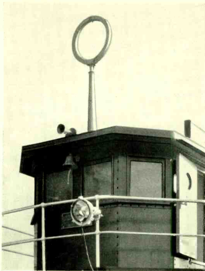
Fig. 2—The loop is mounted in a water-tight aluminum casting, which is supported by an aluminum pedestal fastened to the deck above the wheel house
