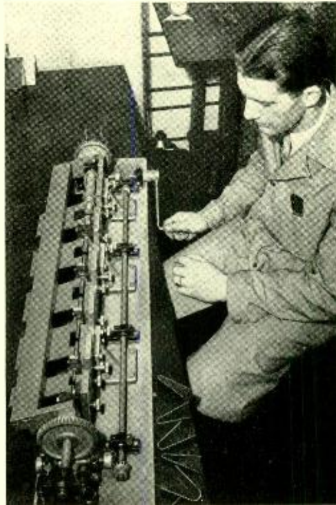
Fig. 3—The mandrel test, in the refined form here being used by H. E. Van Siclen, is a valuable means for determining the flexibility and adhesion of a finish
