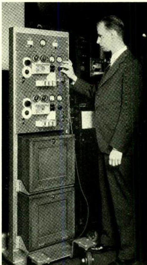
Fig. 4—The new amplifier for use with the rapid record oscillograph, being operated by A. E. Melhose
