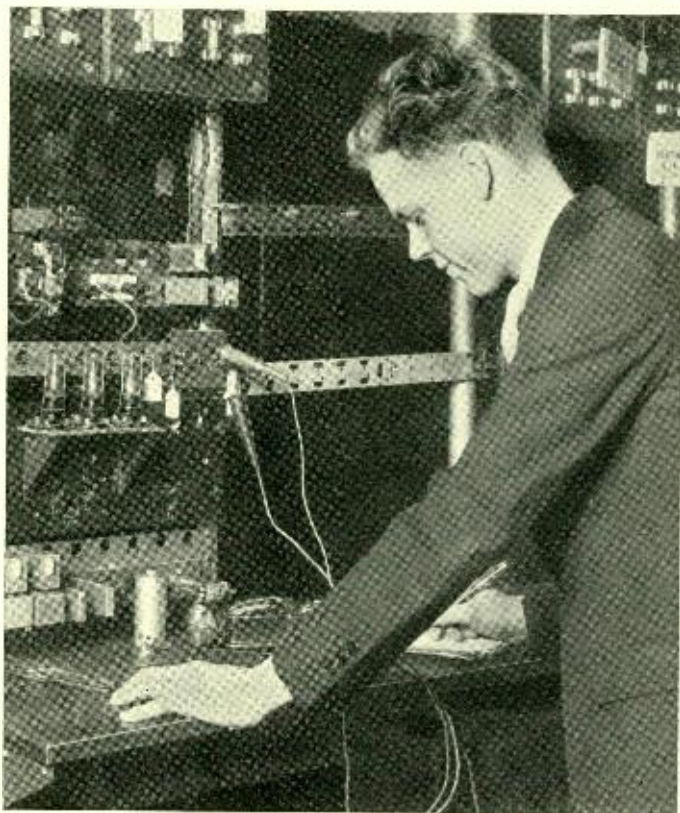
Testing a vacuum-tube circuit designed to transfer the load from the main ringing machine to a second machine in the event of low or high voltage at the ringing panel or upon failure of a brush in the ringing machine. Readings being taken by E. E. Helin of the Equipment Development section of the Systems Department
