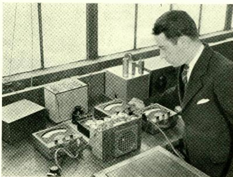
Laboratory measurements being made by J. J. Scanlon of Special Products Development on ultra-high frequency police car radio receiver which covers a frequency band from 30 to 42 megacycles.
