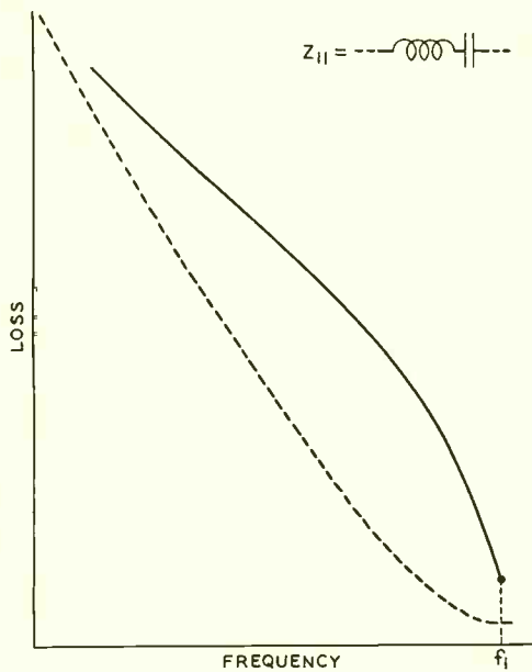
Fig. 8—Loss characteristics obtained by forming a series resonance circuit
