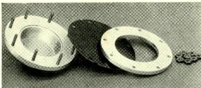
Fig. 1—Water vapor passes from the interior of the aluminum cell through the rubber sample into a drying agent outside
