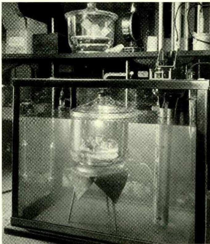
Fig. 2—The temperature is held constant during a diffusion test, often by keeping the cells in a desiccator immersed in a water bath
