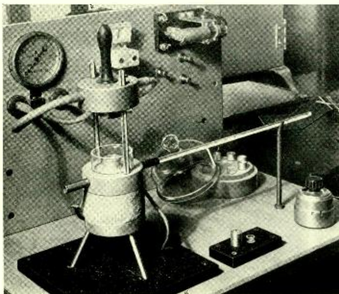
Fig. 1—In a microsublimation chamber designed in these Laboratories, small quantities of volatile solids can be sublimed at controlled temperature and pressure directly onto a microscope slide
