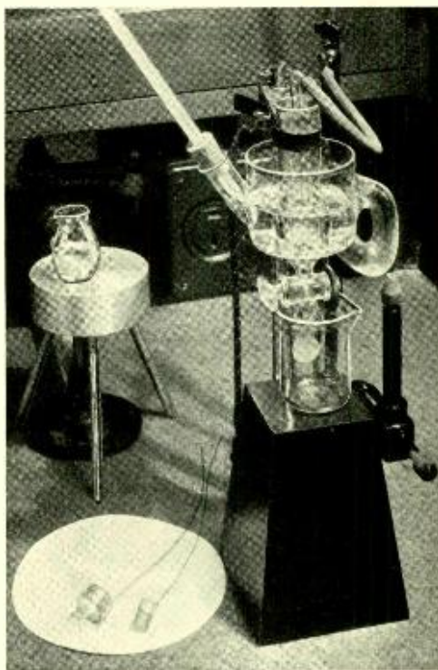
Fig. 4—With this electrolytic cell, as little as one milligram of metal may be precisely determined
