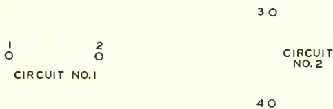
Fig. 2—Between two circuits whose wires are arranged in this configuration no direct crosstalk will take place
