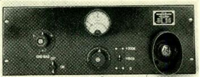
Fig. 2—On the 203C Panel the key and dial in the center are adjusted until the needle deflects to half scale once every ten seconds when measuring program energy levels
