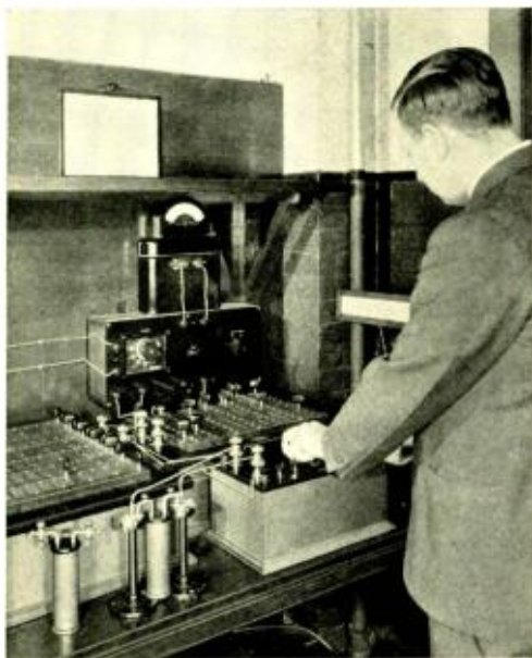
Fig. 5—The primary d-c resistance bridge showing the Bureau of Standards type of resistance standards in the left foreground
