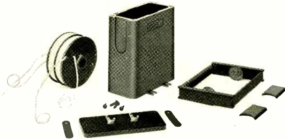
Fig. 1—Coils for precision filters are wound in two sections and then placed in a rectangular container of moulded material
