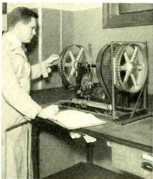
Fig. 4—Abrasion testing machine for wire braids
