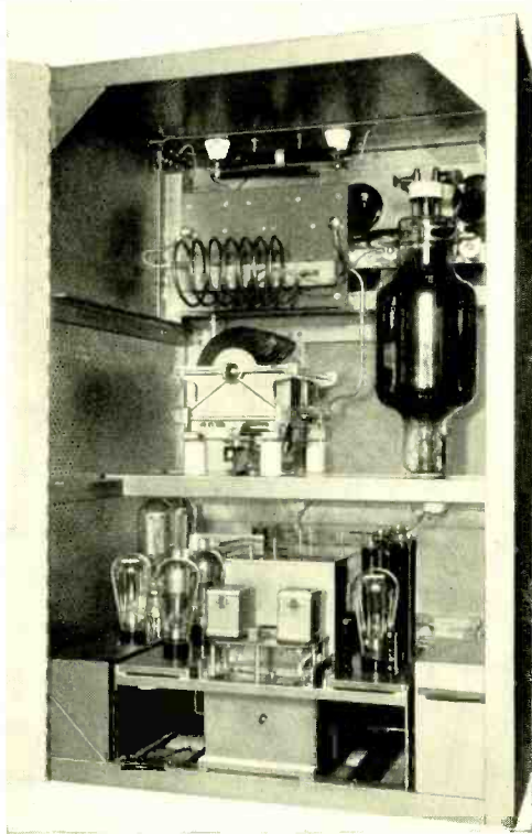
Fig. 1—One of the features of the D-95539 transmitter is the grouping of all low-power radio frequency equipment on a removable frame in the middle at the bottom
