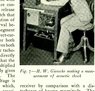
turbance of known magnitude. The apparatus, given schematically in Figure 6, is shown in its actual appearance in Figure 7.
