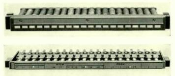
Fig. 1--(above) Until recently the common busy-indicator for toll lines has been the 42-A magnetic signal. Fig. 2--(below) In the new busy-signal strip a 1/16-inch translucent spot on the designation strip is illuminated by the newly developed E-1 lamp
