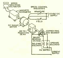
Fig. 4—Duration of disturbance is controlled by a motor-operated device which accurately times by .1 second intervals
