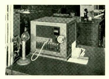
Fig. 3—Turret for test supervisor's private desk with No. 92 jacks mounted at one side
