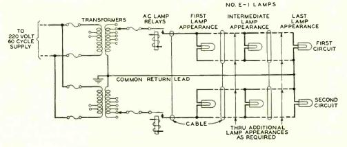
Fig. 4—Typical a-c. busy lamp multiple arrangement [468]
