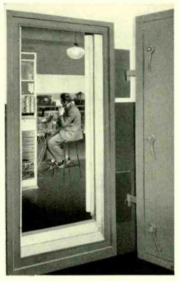
Fig. 4—A cross talk measurement being made in one of the sound-proof rooms
