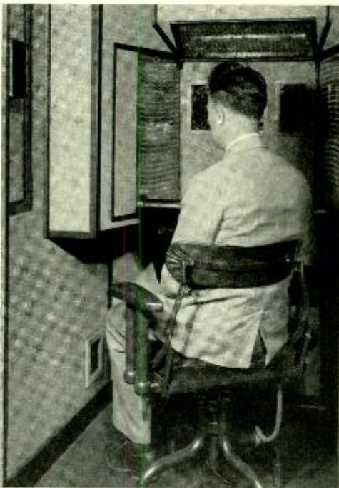
Fig. 1—The two added caesium-oxygen cells appear on either side of the opening through which the television image is seen
