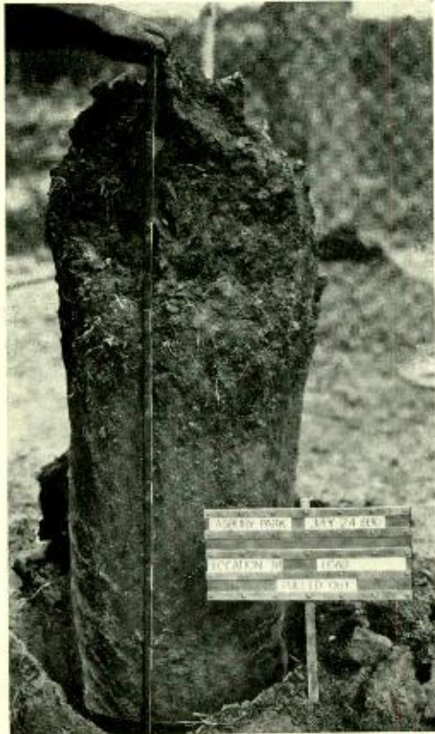
Fig. 6—Sometimes, in pulling out, the anchors would eject large cylinders of soil
