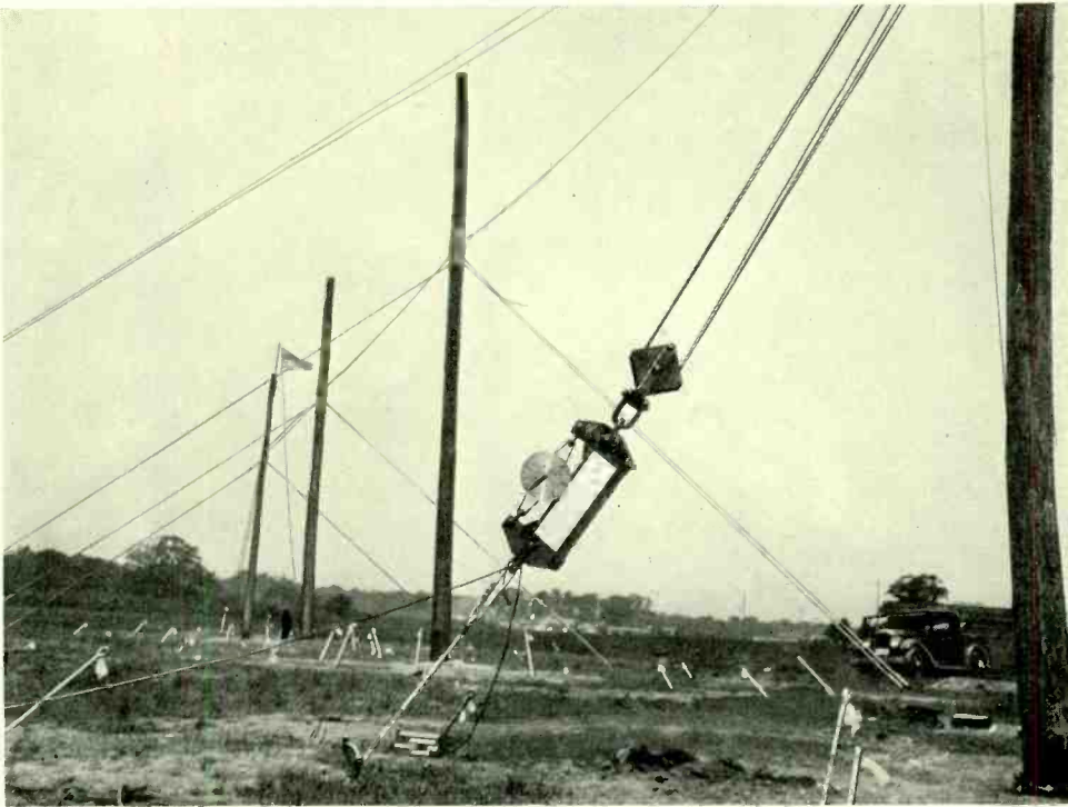
Fig. 2—The dynamometer linkage was fastened directly above the anchor rod
