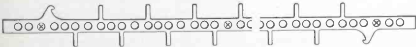
Fig. 2—One of the punchings that compose a panel bank. Three types are used on each bank: one each for the tip, ring, and sleeve terminals. They are all alike except for the location of the terminals and soldering lugs
