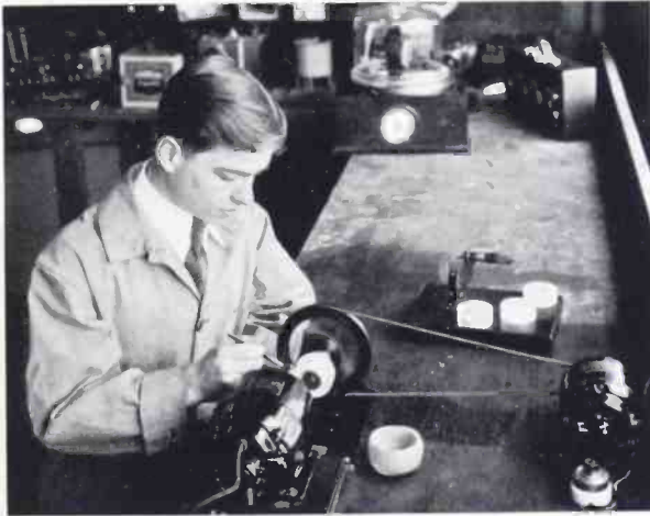
Reducing the diameter of a quartz ring used for a crystal oscillator. Carborundum in the form of paste and applied with a brush is used, in this instance by George Hecht in the Canal Street laboratories of the Research Department
