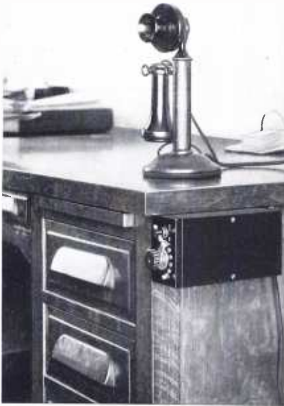
Fig. 1—In an installation of the No. 23-A Amplifier, only the control equipment need be mounted near the telephone
