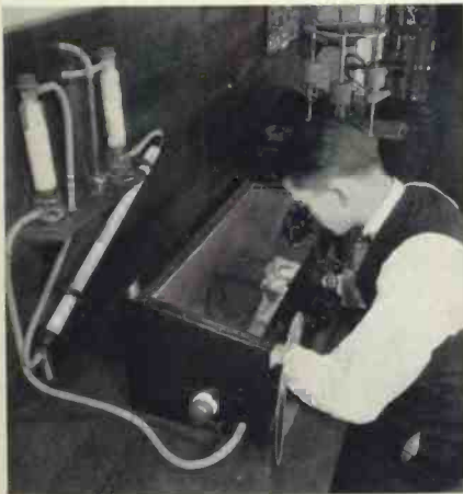
Assembling a condenser microphone in a dust-proof chamber to prevent dust or other foreign material from entering any of the inner chambers of the device. The assembly work is performed by I. H. Baker
