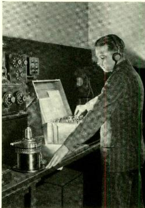
A section of the magnetic research laboratory. E. A. Nesbitt using the Kelsall permeameter for measuring permeability
