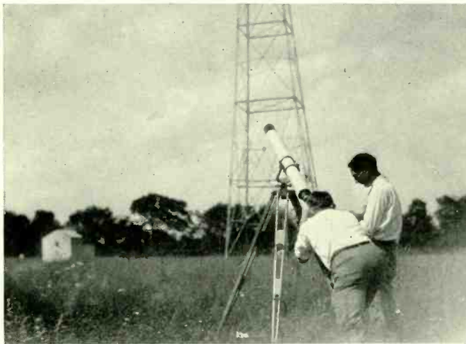
Not star-gazing, but engaged in the serious business of measuring antenna currents, are these two engineers at our Whippany laboratory. When W. N. Mellor calls off the reading of an ammeter suspended in the antenna, E. F.
