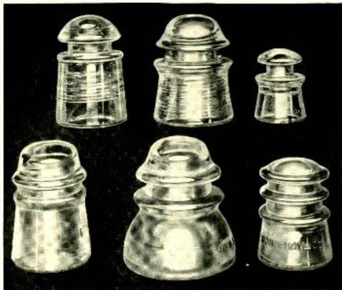
Above, carrier-current insulators, of "low-loss" glass; left to right: CS, CW, CM. Below, non-carrier-current insulators, of soda-lime glass; left to right: Toll line, DP, Exchange
