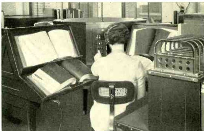
Fig. 2—Directly in front of the operator is the key panel and all around her are the various directories to which she may refer by merely turning slightly in her chair
