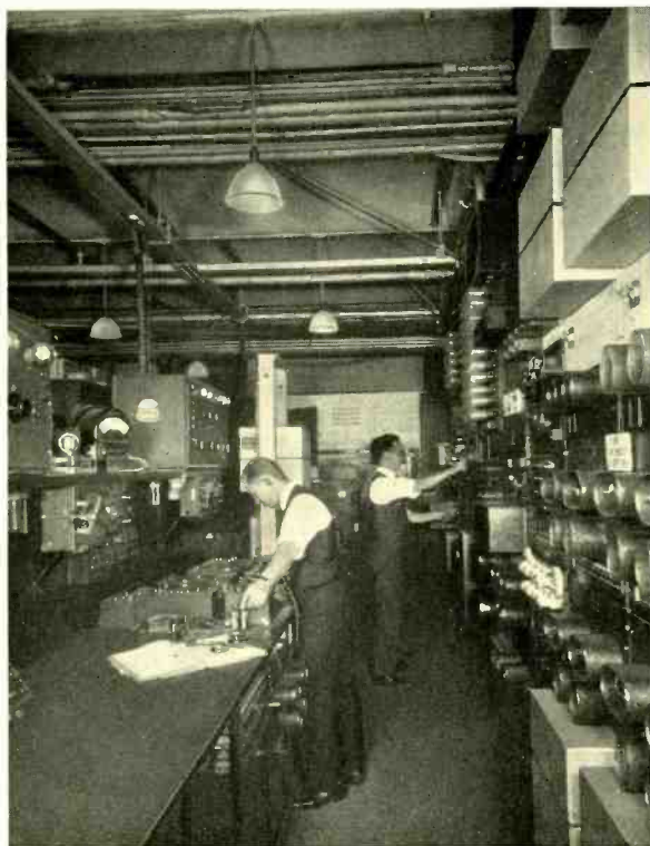
Fig. 9—In this part of the toll circuit laboratory, repeaters for a three-channel carrier system are tested
