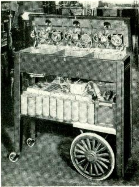
Fig. 3—The raised cover of the amplifier discloses the copper lining that serves as a shield
