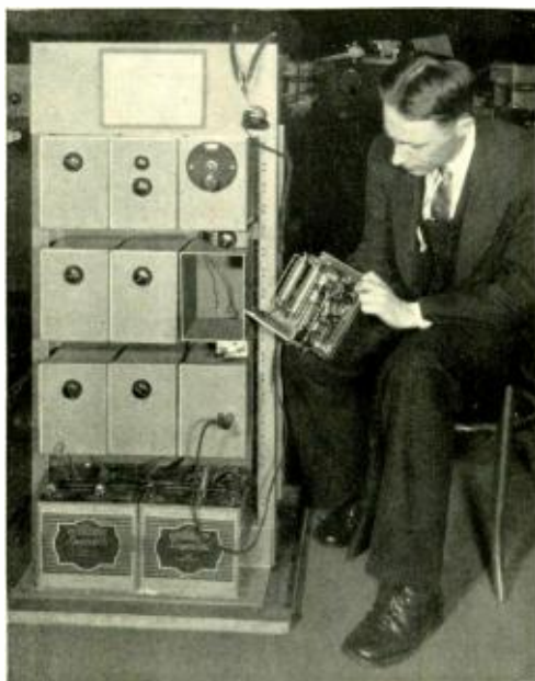
Ship-to-Shore Radio Receiver for use on the S.S. Leviathan
