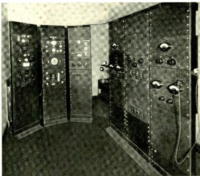
Fig. 2—The Master Reference System of the Bell System, with its associated calibrating equipment. At the right are the transmitter, line, and receiver; at the left are the oscillator, thermophone, and voltmeter and volume-indicator
