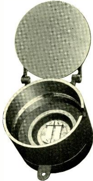
Fig. 4—Thermophone chamber, showing the thermal elements consisting of two strips of gold leaf
