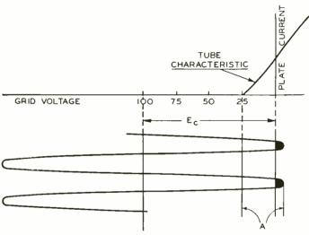
Fig. 3—Production of carrier-frequency oscillations by the oscillator-modulator tubes
