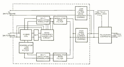
Fig. 1-Equipment symbolized inside the dotted lines is that for the D-1 System
