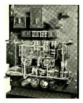
Upper panel carries signalling apparatus of the D-1 Carrier System; lower panel carries, on the side shown, the demodulator circuit
