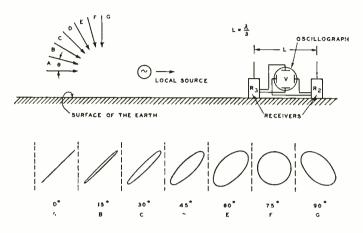
Fig. 2—Arrangement of apparatus for detecting verticalplane angles
