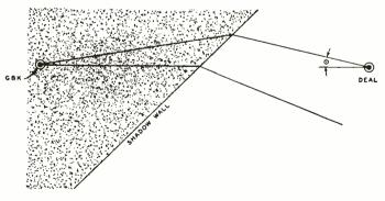
Fig. 3—Suggested way in which the shadow wall affects the receiving angle
