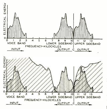
Fig. 4—Above, the location on the frequency spectrum of input and output currents of the modulator; below, how the band-pass filter eliminates all but the lower side band
