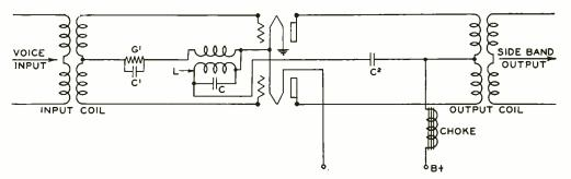
Fig. 2—Modulator circuit of the D-1 System
