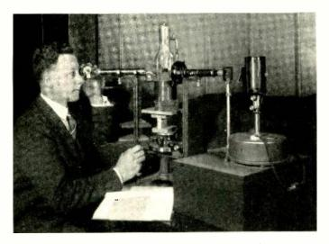
Mr. Johnsrud operates the polariscope, by which the thickness of very thin rubidium films was measured
