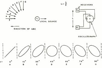
Fig. 1—Arrangement of receivers and local oscillators for determining horizontal-plane angle of reception
