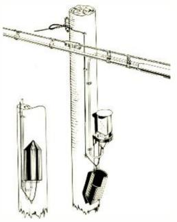
Fig. 3—Method of mounting No. 8 type terminal on telephone pole
