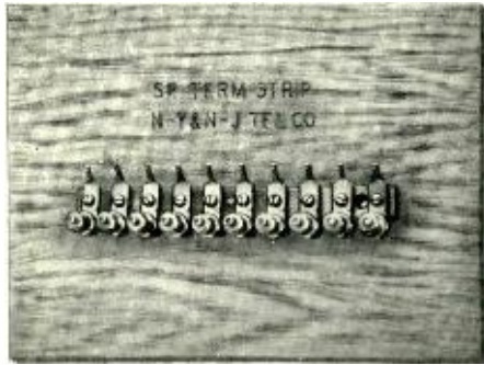
Fig. 1—An early terminal strip, drawn from an old photograph. This was probably used at a switchboard
