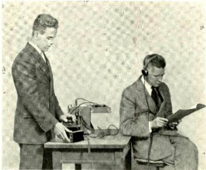
How the 42-A Test Set and the 3-A Audiometer are used to detect deafness is demonstrated by J. A. Battle and W. L. Betts
