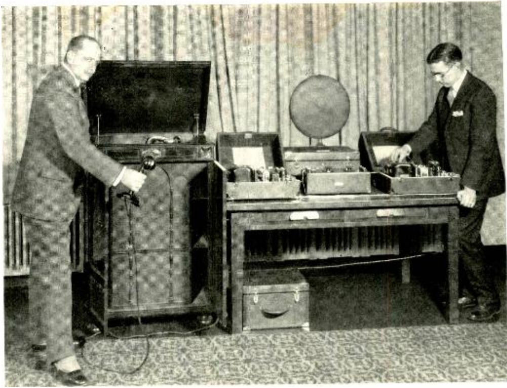
S. P. Grace and L. W. Dacey illustrate the method of using a stage set-up of speech-inversion apparatus
