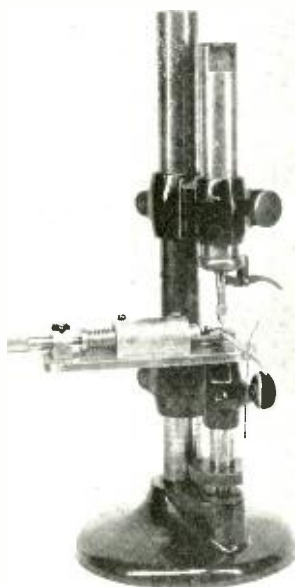
This adaptation of the minimeter gauges fitting to a ten-thousandth of an inch
