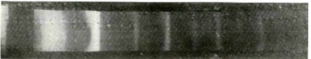
FIG. 5—Diffraction pattern for a piece of 75% iron 25% nickel hammered to a thin strip. X-rays of molybdenum principally of wave length 0.708 \times 10^{-8} cm. Photographic film bent over a quadrant of cylinder. Pattern shows body-centered cubic arrangement with edge of cube 2.90 \times 10^{-8} cm. and also shows that the individual crystals are very small
