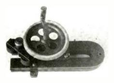
Watson's Hand Generator Used with polarized ringer
