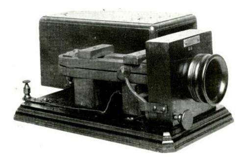
Watson's "Thumper" Number 22 of first series manufactured. The small hammer strikes rear edge of diaphragm when button is pressed
