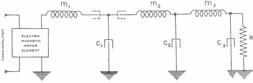
Fig. 2. Schematic of Electrical System Analogous to Recorder
