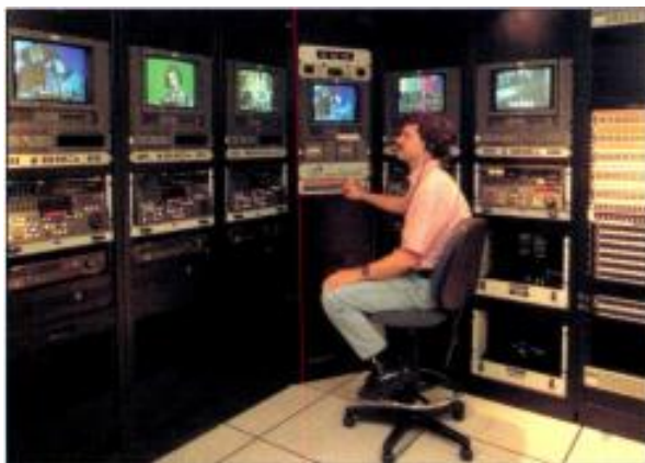
The Digital Betacam control room supports feeds from other stages on the lot.
