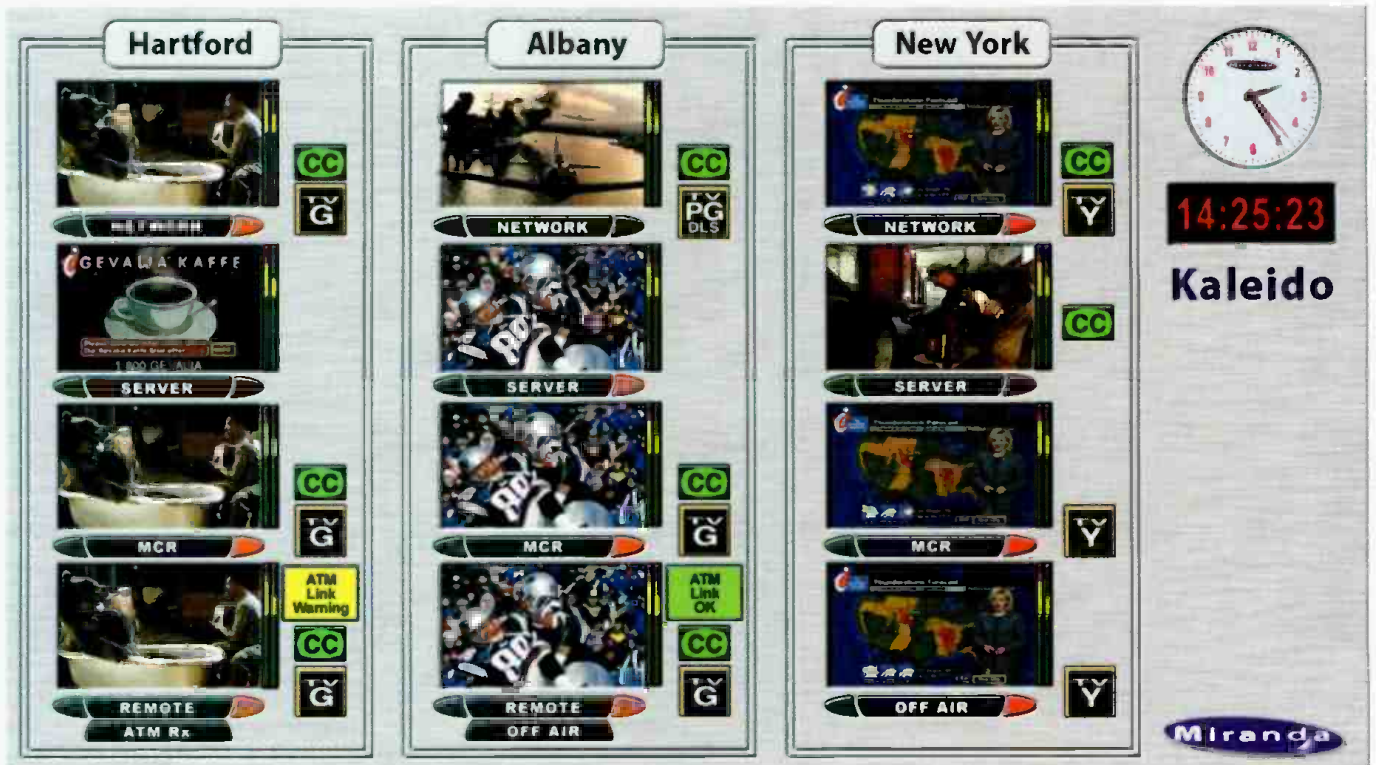
Miranda's Kaleido G2 software allows a technician at a centralcasting hub to monitor and control what's happening at multiple stations.
