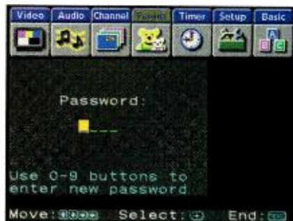
Parents can specify which content ratings will activate the V-chip to block out programs. Access to the chip's programming screen can be password-protected.
