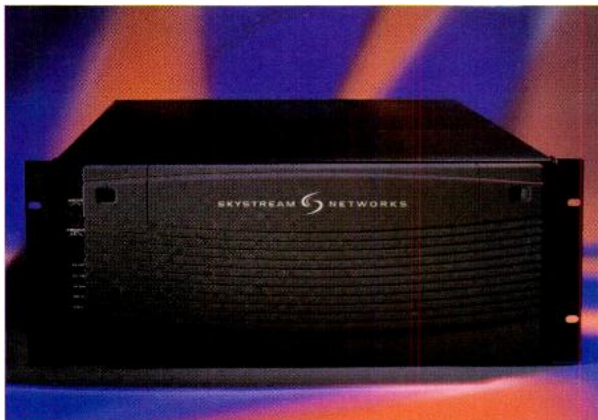
SkyStream Networks' media router, marketed by Harris under the DataPlus brand, can be used to insert IP packets into an MPEG-2 DTV stream. Granite Broadcasting is using it to broadcast Internet content in the San Francisco market.
